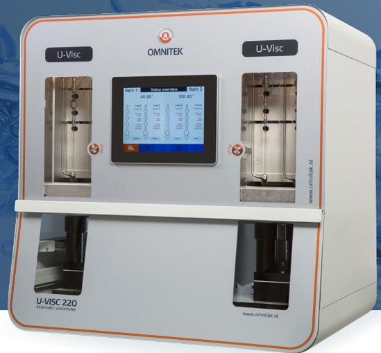
"The U-Visc viscometry system was designed with full ASTM D445 compliance in mind, combined with low solvent consumption, high unattended throughput, ease of use and reliability".
